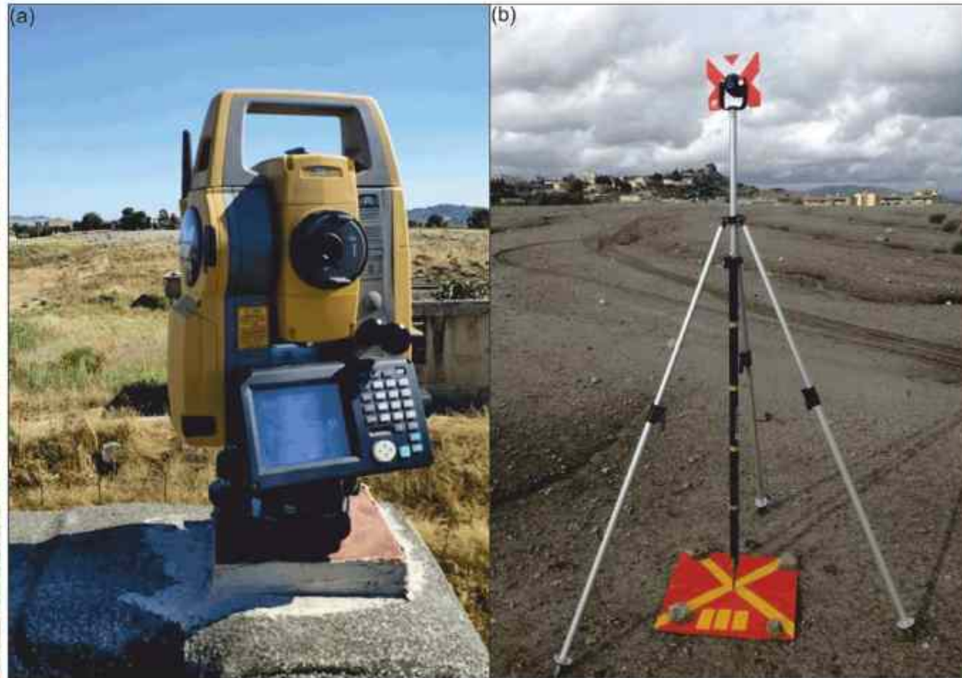
Polar method using total station
