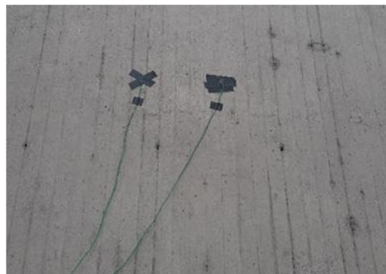
Outside heat flux measurements
