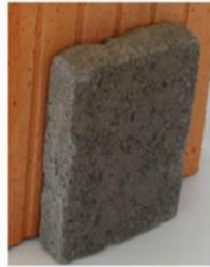
Silica aerogel based thermal mortar – methods of façade wall application
